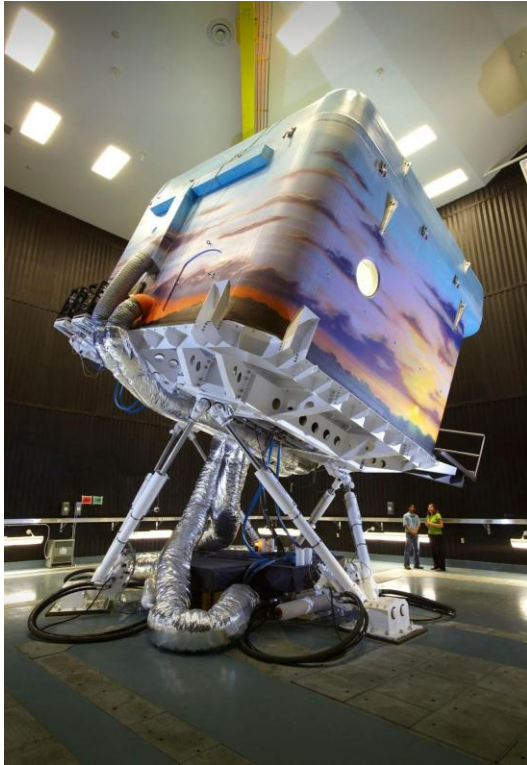
Figure 1: CEAL 6-axis motion base. Pictured is the hydraulic based motion system, with interchangeable payload.
