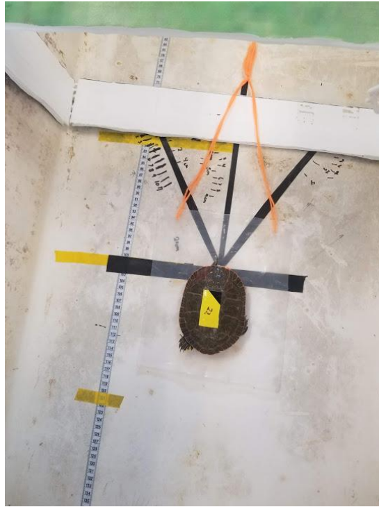
Figure 19: Second set of experimental trials using Western Painted Turtle, Chrysemys picta bellii , cadavers testing the affect of turtle orientation ( 60^\circ , 90^\circ , 120^\circ ) on detection success. The pass-through antenna is shown with a sub-adult, Chrysemys picta bellii cadaver on a sheet of vapor barrier, ready to begin trials with an internal tag facing the antenna at a 90^\circ angle.
