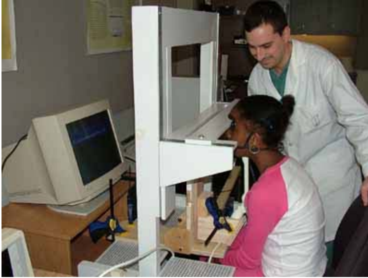
Figure 14. The subject is seated and the head is stabilized in the CHASE apparatus.
