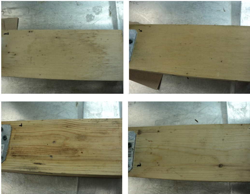
Fig. 12: Comparison between glycerol borate treated(left) and copper borate treated (right) joints (Top- 8 weeks, Bottom- 15 weeks)
