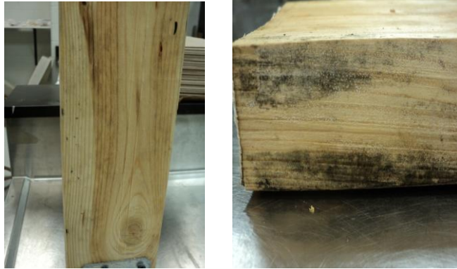
Fig. 11: Treated (left) & untreated (right) parts of joints after 15 weeks(Top - copper borate treated & Bottom - glycerol borate treated).
