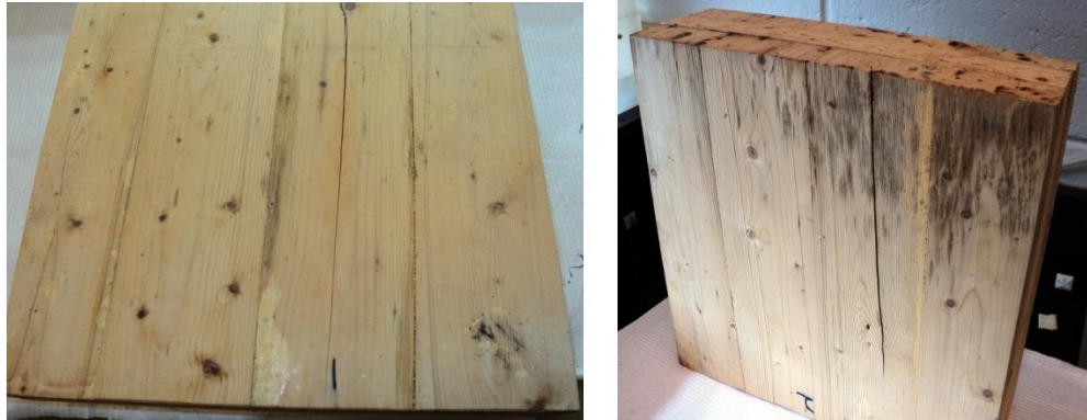
Fig. 16: CLT panel after exposed to extreme condition in two position: left - horizontal, right- vertical.
