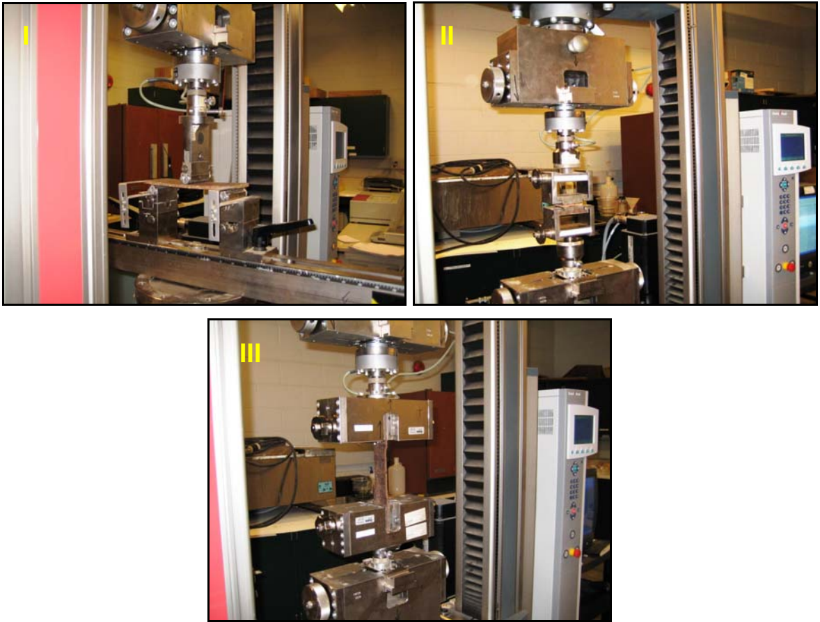
Figure 5.4: Mechanical testing of barkboard (I. Static Bending, II. Internal Bond, III. Tensile Strength).
