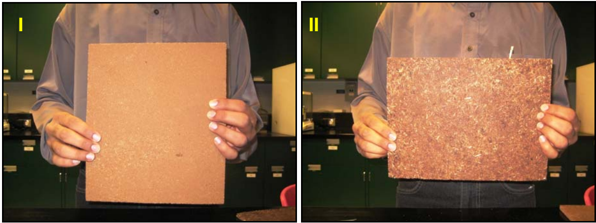
Figure 4.4: Barkboards made from fine (I) and mixed (II) size particles.
