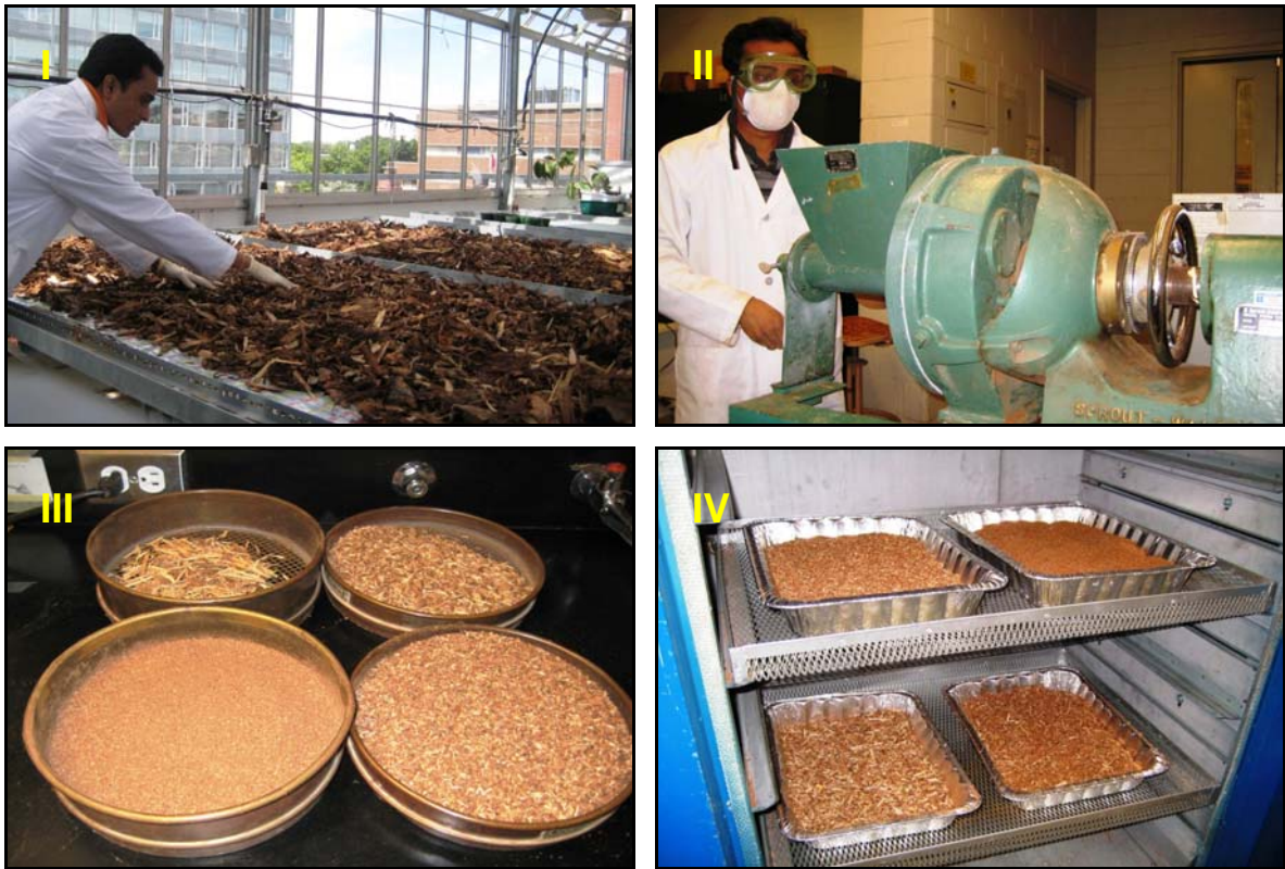
Figure 4.1: Preparation of bark for board production. (I. Air-drying, II. Grinding, III. Screening, IV. Oven-drying)
