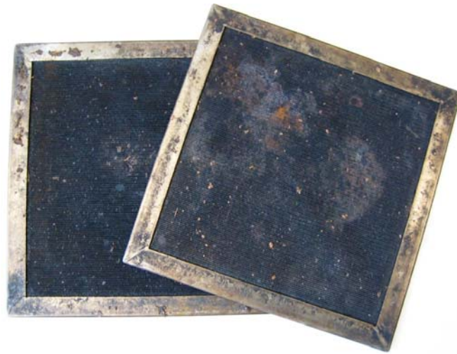
Figure 4.6: Special caul screens used during the hot pressing of boards to control the core gas pressure.
