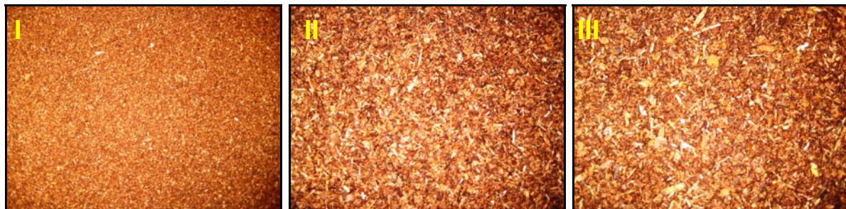
Figure 5.1: Three different particle sizes were considered in the experimental design of barkboards (I. Fine, II. Medium, III. Coarse).
