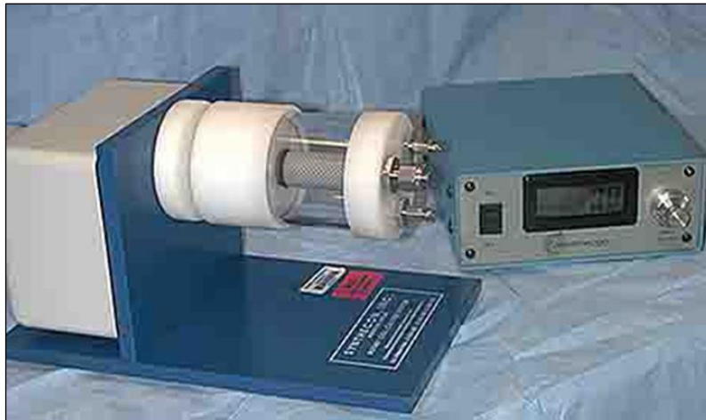
Figure 4-1. Rotary Cell Culture System (RCCS) utilizing a Slow Turning Lateral Vessel (STLV) (Synthecon Inc.)
